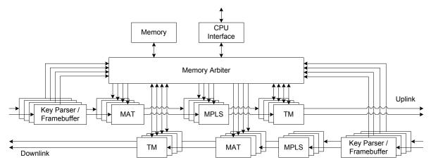
Fig. 2. Internal structure of the MATMUNI system with serially ordered functional modules
