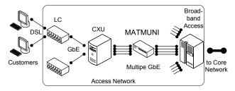
Fig. 1. Structure of an access network and logical location of MATMUNI
