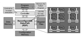
Vulcan's computation power and flexibility is due to its RDP (Reconfigurable Data Path) module which is a reconfigurable network of processing elements (PE). Additional calculation units are present for more demanding arithmetic computations. The controller is responsible for fetching instructions, reconfiguring the RDP and handling flow changes (e.g. branching).
