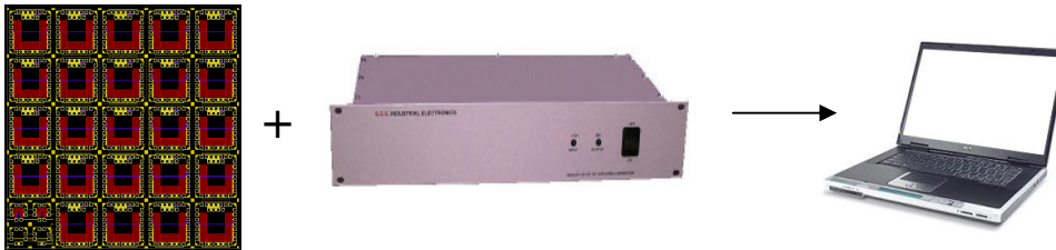
Fig.3 Modular test chip and high current driver and measurement unit
