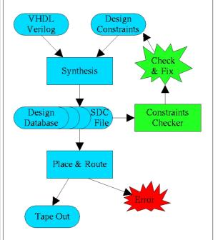
The Chip Design Constraints Checker can easily be adapted to almost every design flow running on Workstation or PC. Tools from the following CAD vendors are supported: Synopsys, Avant!, Magma and Cadence. Other vendors on request.
